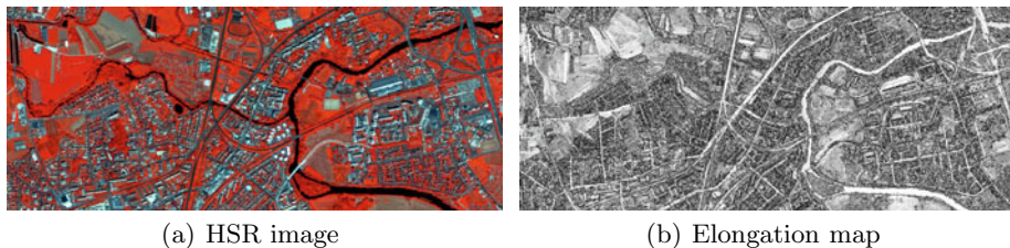
Fig. 4. Elongation map computation. (a) HSR image with a spatial resolution of 2.4 m (QUICKBIRD, © DigitalGlobe Inc.). (b) Corresponding elongation map (elongated structures in light grey, non-elongated ones in dark grey).
